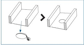
**2.** Select a desired method for cutting the hole. Do not cut the hole bigger than the plate opening.
