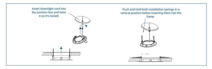
4. Connect the power cords and insert the downlight into the frame.
