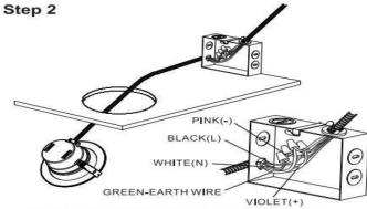
Connect AC and Dimming wires correspondingly as shown in picture
